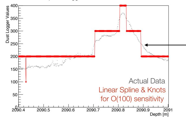
Separated by mm in depth, yet logger would produce drastically different values. If we 'know' that there are smoothly varying features we can proceed to smooth the data
