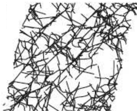
Figure 10.12: Network configuration at strain angle \Gamma = 0.24 from a finite element simulation(?). Percolations of stretched filaments appear that connect the top and the bottom of the cell along a 45^\circ direction. (Figure taken from Onck et al., Physical Review Letters , 2005, Ref. [88]).
