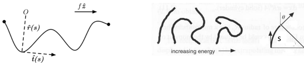
Figure 34: A homogenous molecule described by: \hat{r}(s) position vector as a function of the L_c where s is a point on L_c . Its unit tangent vector: \frac{d\hat{r}(s)}{ds} = \hat{t}(s) with respect to line segment (36)- As thermal energy increases the molecule can be in more coiled configurations (35).
