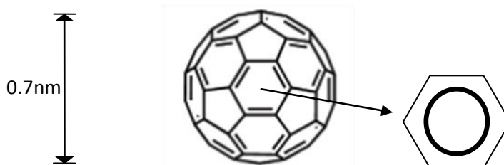
Figure 22: C_{60} a symmetric 3 dimensional closed cage molecule comprised faces of 20 hexagons and 12 pentagons, and a carbon at the vertexes (22) (54). Black circle in the close up illustrates an aromatic ring.
