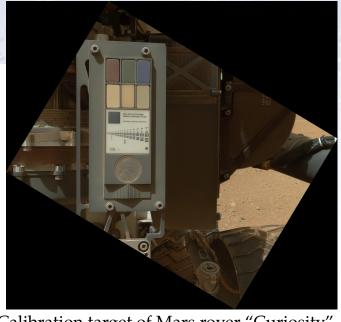
Calibration target of Mars rover "Curiosity"
