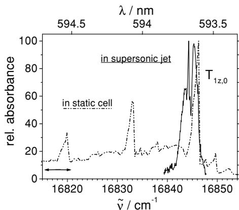
FIG. 5. (A) Comparison of the unresolved rotational structure in the region of the  $T_{1z,0} \leftarrow S_{0,0}$  transition of jet-cooled PT “—” (A-type envelope) and of PT in a static cell “---,” measured with the cavity ring-down method. The horizontal brace indicates the region where  $T_{1(xy),0} \leftarrow S_{0,0}$  transitions would be expected.
