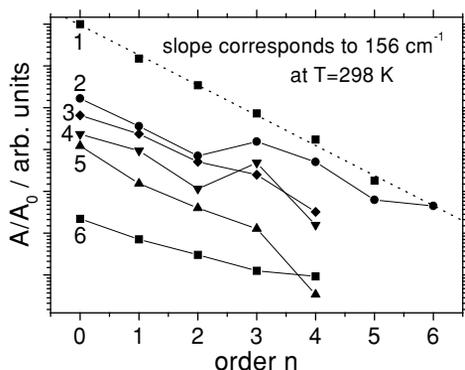
**FIG. 3.** Semilogarithmic plot of the relative absorbances of lines of 6 different harmonic sequences versus their order in the respective sequence. The dotted line represents a monoexponential function fitted to the datapoints. Origins of the sequences are 1:  $16\,846.4\text{ cm}^{-1}$ ; 2:  $17\,231.6\text{ cm}^{-1}$ ; 3:  $16\,849.8\text{ cm}^{-1}$ ; 4:  $16\,810.7\text{ cm}^{-1}$ ; 5:  $17\,307.3\text{ cm}^{-1}$ ; 6:  $16\,995.2\text{ cm}^{-1}$  (compare Table 1).
