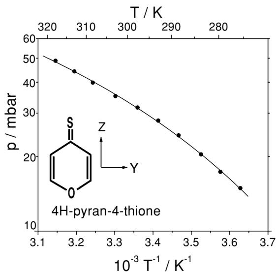
FIG. 1. Temperature dependence of the vapor pressure of 4H-pyran-4-thione. The solid line was calculated with the Antoine Eq. [1] using the parameters  $A = 2.529$ ,  $B = 94.609$  K, and  $C = -205.977$  K, which were calculated in a nonlinear least-squares fit.
