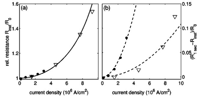
FIG. 3. Comparison of the measured heating of wires of different widths [5  $\mu\text{m}$  ( $\nabla$ ), 50  $\mu\text{m}$  ( $\bullet$ )] to the two models (solid and dashed lines; no fitting parameters used). (a) The fast heating process depends solely on the current density. (b) For the slow process, the wider wire exhibits a larger temperature increase at equal current density.
