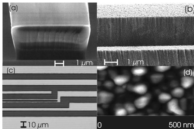
FIG. 1. Microscope images of chip details during and after the fabrication. (a) SEM picture of the resist structure. Its thickness is 4.5  $\mu\text{m}$ , the undercut is 0.6  $\mu\text{m}$ . (b) SEM image of a typical fabricated wire. (c) 1, 5, and 10- $\mu\text{m}$ -wide gold wires on a fully fabricated chip. (d) AFM picture of the gold surface. The grain size is 50–80 nm.
