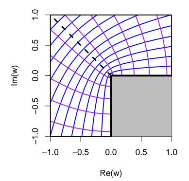
The real and imaginary parts of a holomorphic (analytic) function in the complex plane,  $f = \psi + i\phi$ , are always harmonic, that is they satisfy the Laplace equation
