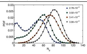
FIG. 4 (color online). Probability distribution function of dislocation density fluctuations corresponding to PFC single crystals sheared at different shear rates. The continuous lines represent the stationary probability distributions predicted by the stochastic model of dislocation number fluctuations from Eq. (6). Numerical values of the model fitting parameters are tabulated below
