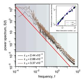
FIG. 3 (color online). Power spectrum of the dislocation number fluctuations  $N_d$  vs frequency f for different strain rates. The red line shows the prediction of the stochastic model Eq. (4), varying as  $C/f^2$  for large f. The inset shows the dependence of C on the mean dislocation number. The error bars in the inset are given along the principal axes of the variation over multiple simulations of the mean of  $N_d$  and C.
