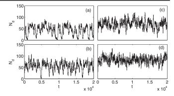
FIG. 2. Temporal fluctuations in the dislocation number for different strain rates. From (a) to (d) the strain rate increases as  $2.78 \times 10^{-4}$ ,  $3.02 \times 10^{-4}$ ,  $3.41 \times 10^{4}$ , and  $3.90 \times 10^{-4}$ .
