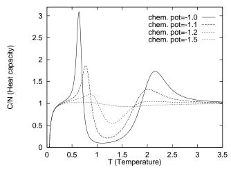
Fig. 2. Specific heat as function of temperature T for the model, with four different values of the chemical potential  $\mu = -(\mathcal{E}_0 + \mathcal{E}_{min}) = -1.0, -1.1, -1.2, -1.5$  and with fixed level spacing  $\Delta \mathcal{E} = 0.2, g = 35$  and system size N = 60. As the chemical potential is lowered, it becomes increasingly difficult to fold, and finally for sufficiently low  $\mu$  the protein stays unfolded.
