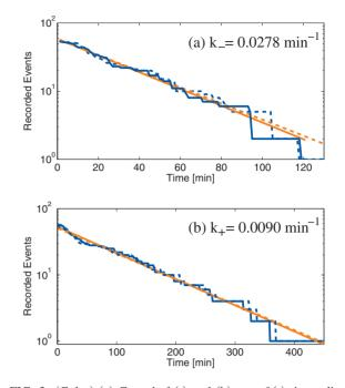
FIG. 3. (Color) (a) Growth  $f_g(t)$  and (b) stop  $f_s(t)$  times distributions on semilogarithmic scales. Blue lines are data and yellow straight lines are the exponential fit. Both for data and fits, continuous lines are the lower estimates and dashed lines are the upper estimates (see text). All fits are of extremely good quality as indicated by the large *R* value,  $R^2 > 0.98$ .
