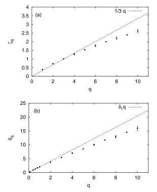
FIG. 2. (a) The exponents  $\zeta_q$  for the velocity structure functions, with selected error bars. The line corresponds to Kolmogorov theory. (b) The exponents  $\delta_q$  for the distance structure functions. The line is adjusted to pass through the value of the first order exponent  $(1, \delta_1)$ .
