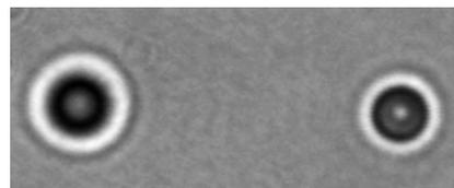
Fig. 2. Microscope picture containing both a bead stuck to the surface (left) and a bead (right) in the optical trap the position of which nearly coincides with the focus of the microscope above the surface.
