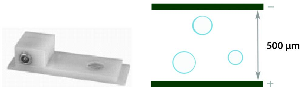
**Figure 2.3:** **Left:** Micro fusion chamber from Eppendorf showing the electric connector and the sample hole with the two electrode wires. **Right:** Sketch of the gap between the two electrodes. The vesicles are shown as blue circles. The anode was on the side of the electric connector of the chamber.
