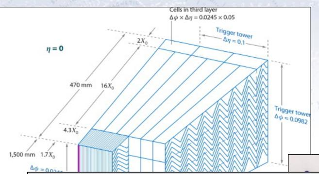
The ElectroMagnetic (EM) Calorimeter records the energy of a shower.
