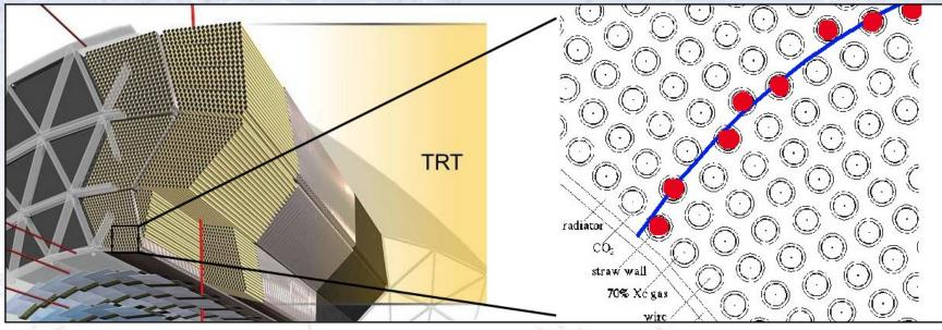
The Transition Radiation Tracker (TRT) records the passage of charged particles. The particles typically pass through 30-35 straws, each giving two signal:
