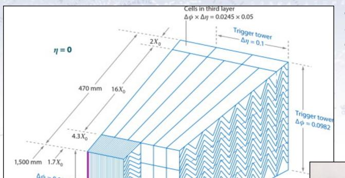
The ElectroMagnetic (EM) Calorimeter records the energy of a shower.
