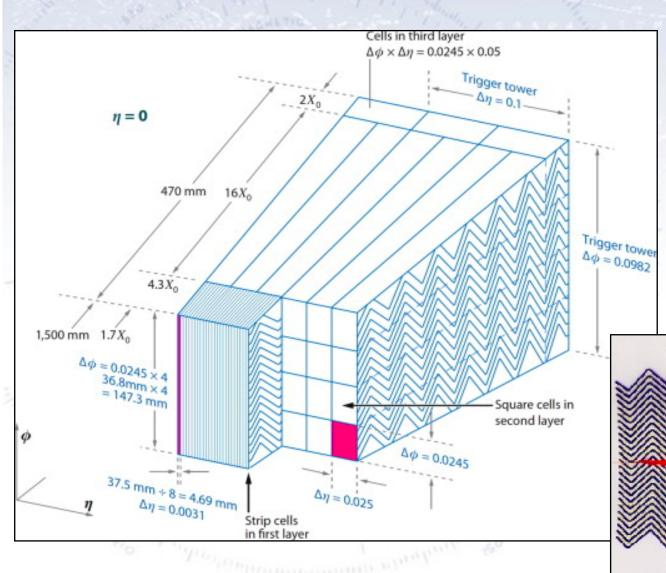
The ElectroMagnetic (EM) Calorimeter records the energy of a shower.
