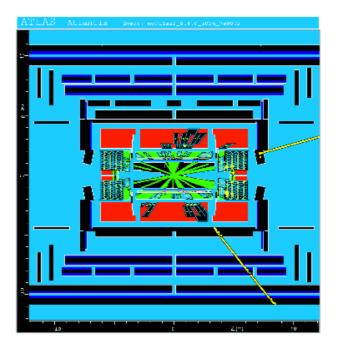
This event from Standard Model ttbar production also has high  $p_T$  jets and muons, and some missing transverse energy.
