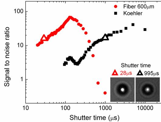
Fig. 3. Signal-to-noise ratio as a function of camera shutter time for illumination by  $600\ \mu\text{m}$  optical fiber (red curve) and Köhler alignment (black curve). The inset shows CMOS images of colloids yielding the same signal-to-noise ratio of 16 at very different shutter times of  $28\ \mu\text{s}$  (fiber illumination) and  $995\ \mu\text{s}$  (Köhler illumination). The intensity of each light source was kept constant during the measurement.
