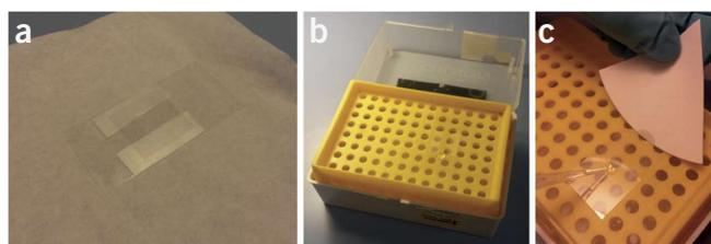
**Figure 5** | Preparation of perfusion chamber. (a) Construction of chamber. (b) The finished perfusion chamber in the evaporation box. (c) Example of how to exchange the medium in the perfusion chamber.
