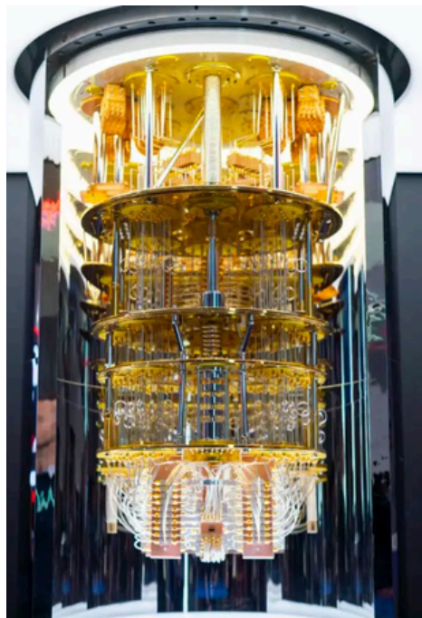
Superconducting Circuit Based Computer (Artificial Atoms)
