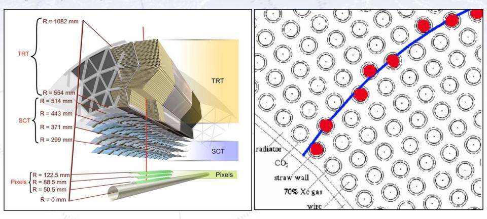
The probability of TR hit (called High-Threshold hit) is about 20-25% for electrons, while it is 4-6% for pions. Given 30-35 hits, this gives a difference.
